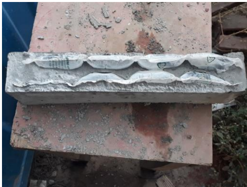
Figure 14 concrete block with insulating air bubble pouches inside
