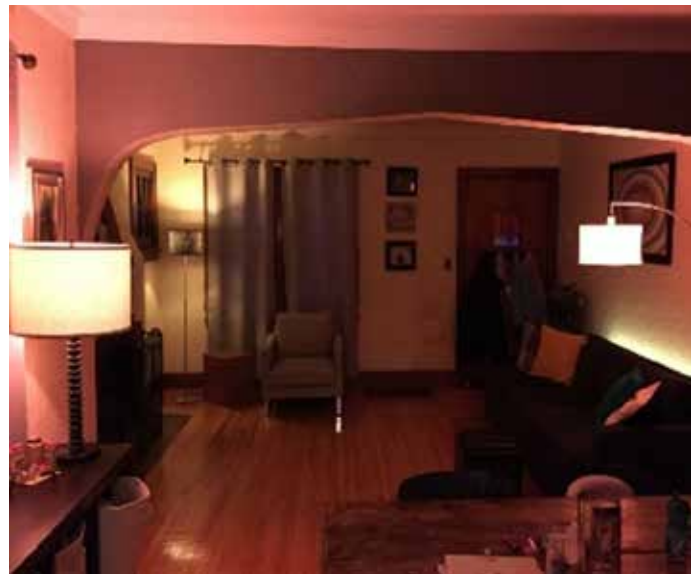
Figure 9: Inadequate arrangement of lighting design to light the living space
