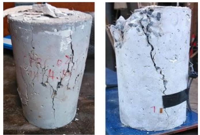
(a) Static failure (b) Impact failure
